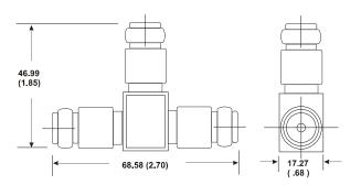
PHASE TRAKING: ±2° nominal between output ports
